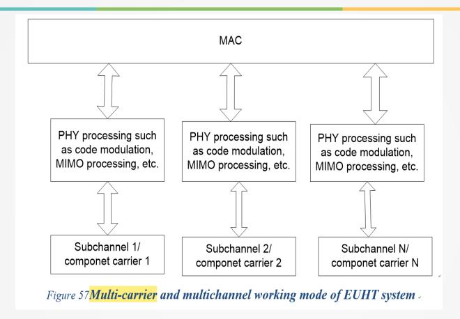
■ As shown by Fig 57 in EUHT specification, spectrum aggregation is defined. Each component carrier is independently processed in physical layer. All the component carriers are processed by a single MAC layer entity.
