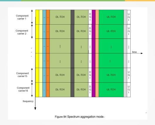
■ In section 8.11, CCH and TCH in each component carrier can be different. In the figure above, there are 16 aggregated component carriers. each CC have its own SICH/CCH/TCH channel respectively, which means the resource allocation and data transmission in time/frequency/spatial domain can be accomplished for each CC independently.
